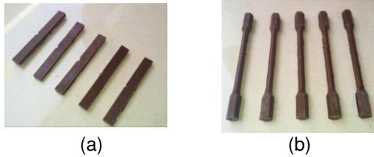
Figure 4. (a) Impact test specimens, (b) Twisting test specimens
