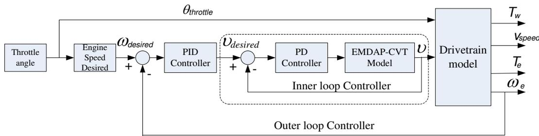
Figure 2. PID controller used for outer loop drivetrain control
