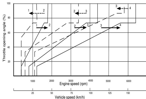
Figure 1. A typical automatic transmission shift pattern
