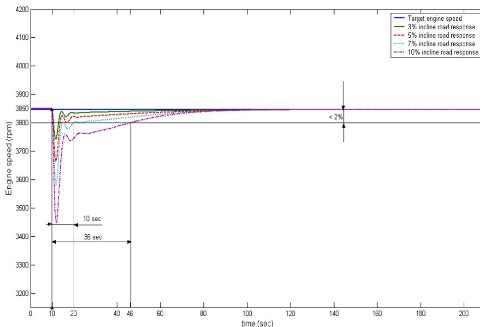
Figure 4. Performance of adaptive ANN controller for constant throttle and various road gradients
