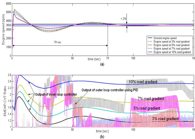
Figure 3. Performance of PID controller as outer loop controller at 80% throttle opening with road gradient variation
