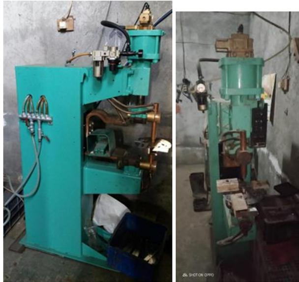
Figure 4. RSW machine 35 kW in capacity
