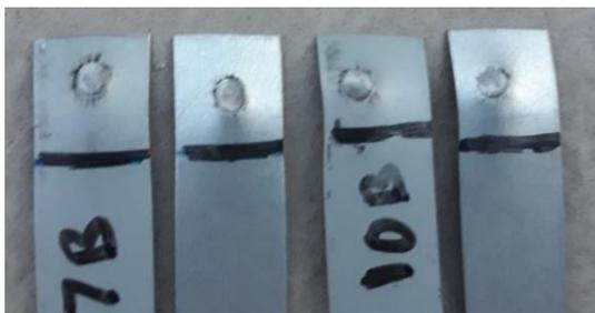
Figure 7. Interfacial Failure Mode
