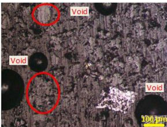
Figure 5. Cross-sectional morphology of polymer-basalt composite with a variation of 60 mesh-75% basalt-1/30 catalyst powder
