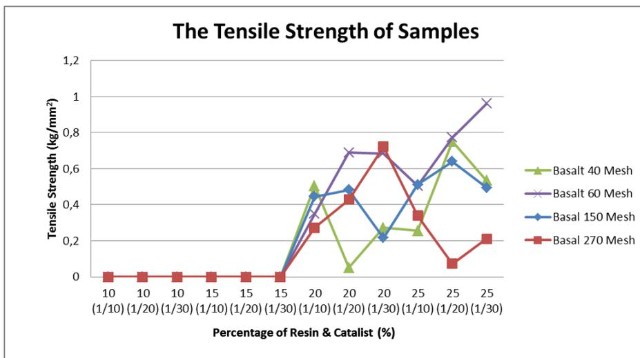
Figure 3. The results of the polymer-basalt composite tensile test
