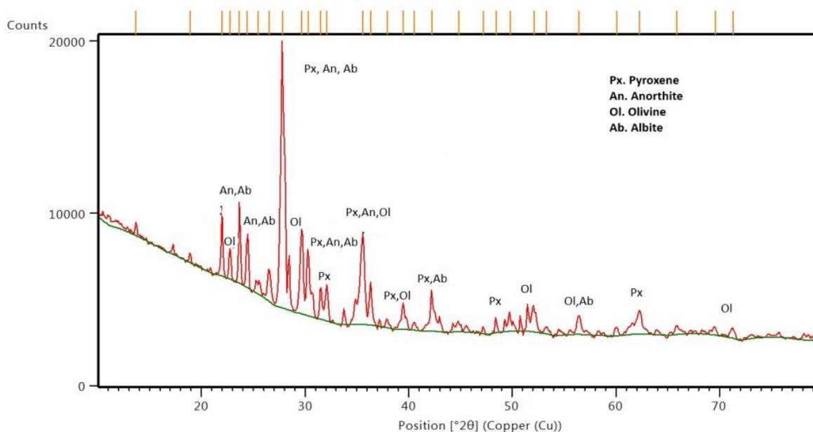
Figure 1. The result of XRD analysis of basalt rock in Sukadana, East Lampung
